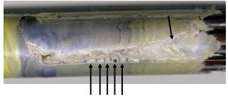
These appear to be partially melted pellets
