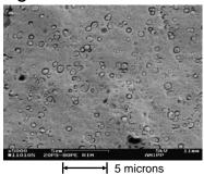
X5000 magnification, shows PS domains ~1 micron and smaller
