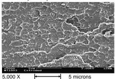
Figure 13: 30 to 60 nm Ceramic Powder, 5%, In PMMA Pellets
