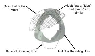
Figure 7: Flat View of Mixer Flood Fed Input
