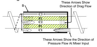
Mixer Flow With Input Below Pumping Capacity of P1 and P2
