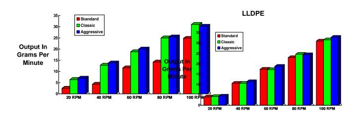
The output from both the "Classic" and "Aggressive" feed throats are much higher than the "Standard" feed throat and both produced stable pressures. This implies that the "Standard" feed throat supplied too little material to the metering section and it was consequently starved and surged.
