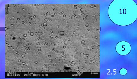
This picture shows minor phase domains of 1 micron from our AFEM mixing screw.
