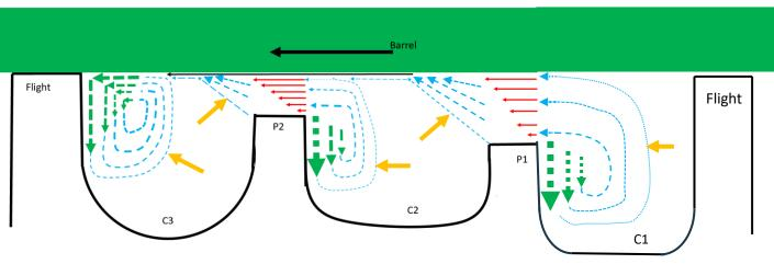
Red Arrows: Simple Shear Aqua: Elongational Flow Green: Adhesion/slowed velocity Orange: The 5 Free Surfaces
