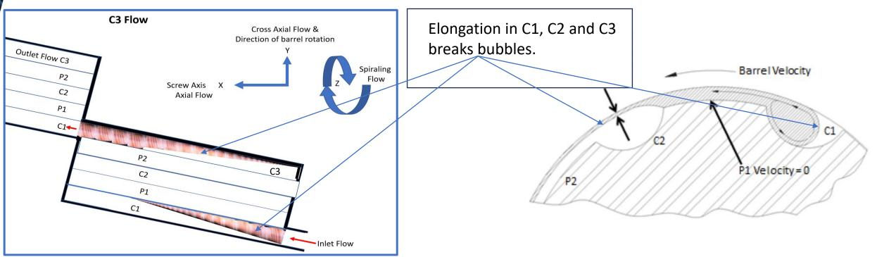
3D mixing is essential so that volatiles are brought to the surface where bubbles can break and gas escape.
