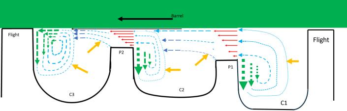
Red Arrows: Simple Shear Aqua: Elongational Flow Green: Adhesion/slowed velocity Orange: The 5 Free Surfaces
