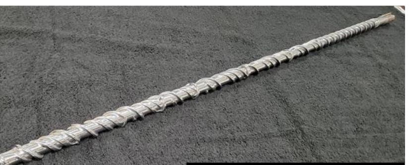
In a starved condition, the entire length of the continuous mixing section can operate at zero pressure for venting through a single vent.
