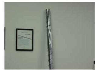
Figure 5. – 2.5" NRM SSE with SFEM Shown
