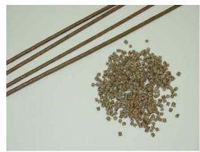
Figure 8. – Compounded RPVC and wood flour mixed throughout the strand with moderate melt strength.
