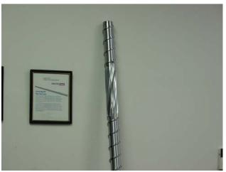
Figure 5. – 2.5" NRM SSE with SFEM Shown
