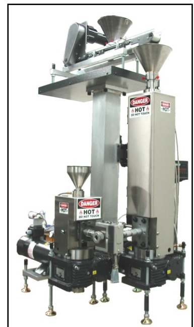
Right: A 50:1 L/D RCP-0500 compounder with (4) Recirculator mixing elements in a coextrusion system with a 24/1 RCP-0250 extruder to make bi-component fibers or rods. An optional starve feeder is shown that increases compounding flexibility.
