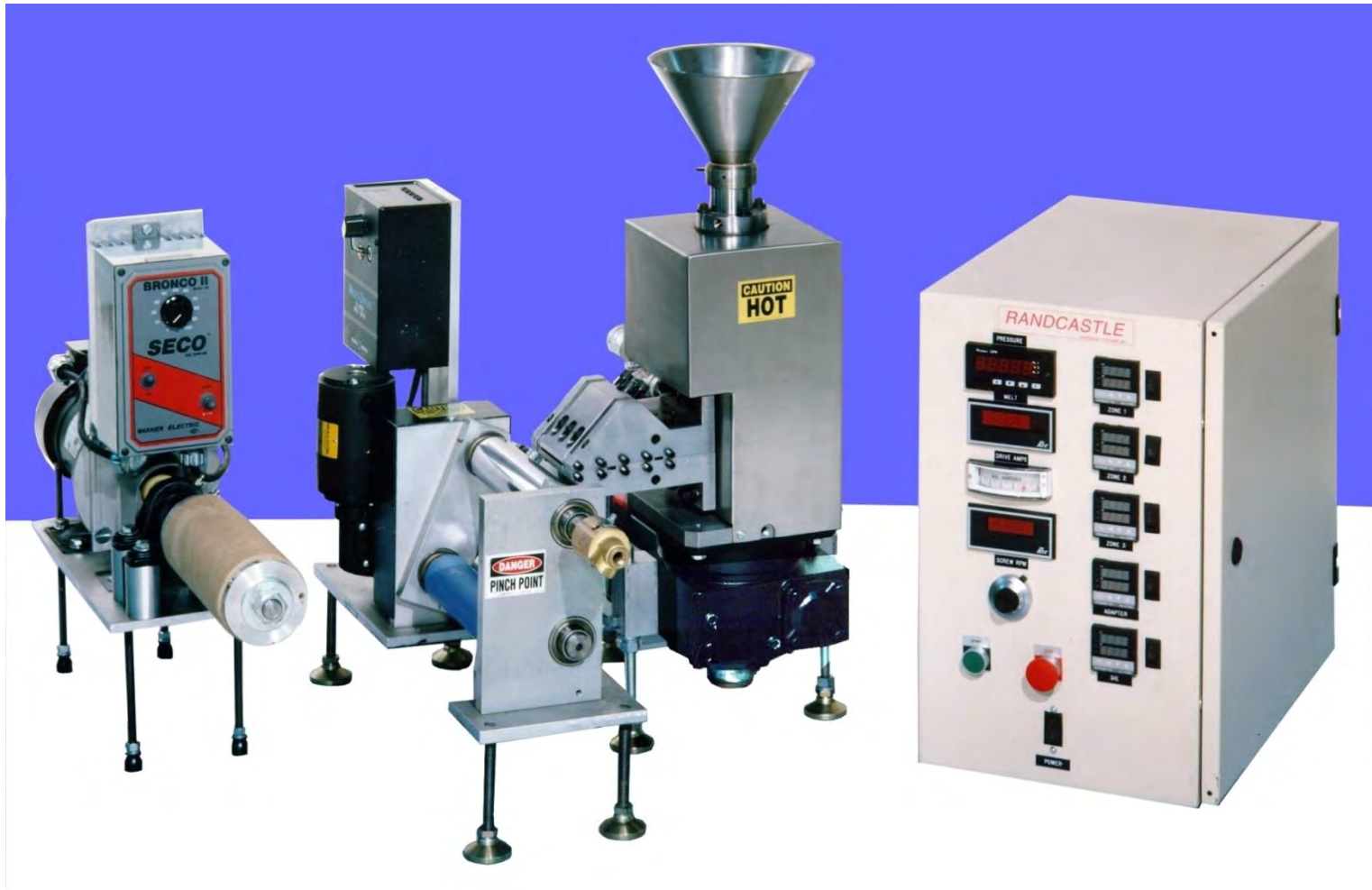
RCP-0375 Microtruder with control panel 2.5 inch strip die, 7 inch chill roll and in-line torque winder.
