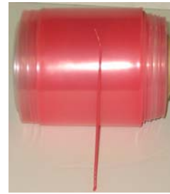
Figure 6. 1% red color concentrate pellets/LDPE showing the film produced using the SSE and rod produced using the micro-batch mixer, both with the SFEM mixing elements.
