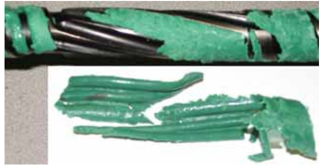
Figure 12. – Screw pull of RPVC and Green color concentrate, second SFEM-II.
