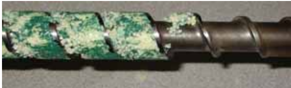
Figure 9. – Screw pull of RPVC and Green color concentrate, feed section.
