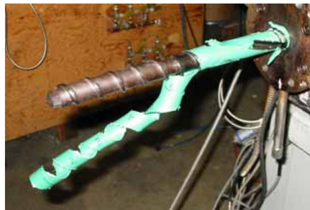
Figure 7. - Screw pull of RPVC and Green color concentrate, metering section and third SFEM-II.
