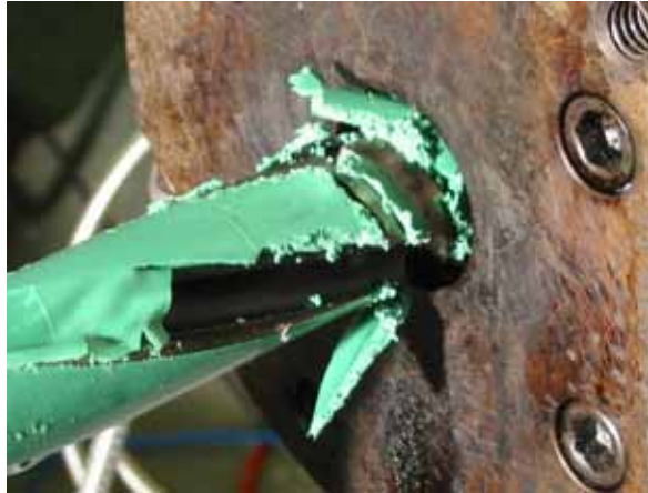
Figure 8. – Screw pull of RPVC and Green color concentrate, third SFEM-II.
