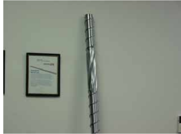
Figure 5. - 2.5" NRM SSE with SFEM-II Shown
