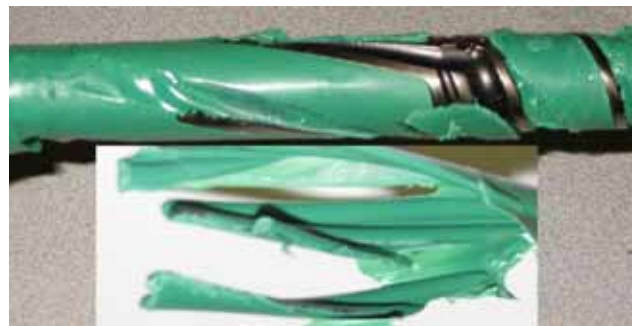
Figure 13. – Screw pull of RPVC and Green color concentrate, third SFEM-II.
