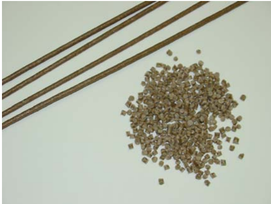
Figure 8. – Compounded RPVC and wood flour mixed throughout the strand with moderate melt strength.
